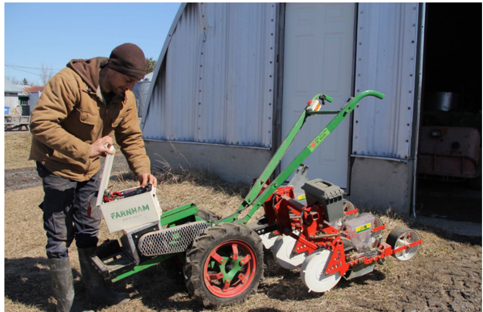
Figure 2: Reid Allaway demonstrating his precision push seeder that he enhanced through a built-in battery to turn into an E-seeder
