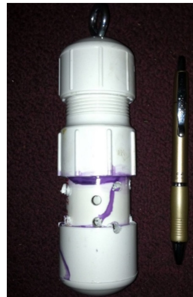
Figure 6. This two-inch PVC pipe can hold liquid or loose bait. Photo by Stephen M. Vantassel.
