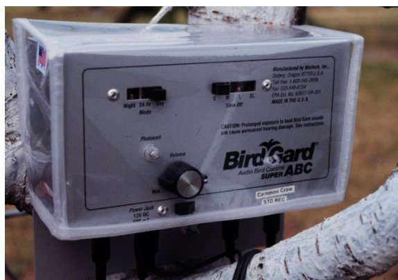
Figure 6. Device using both bird distress calls and raptor calls to deter birds from fruit crops. Image by Paul D. Curtis.
