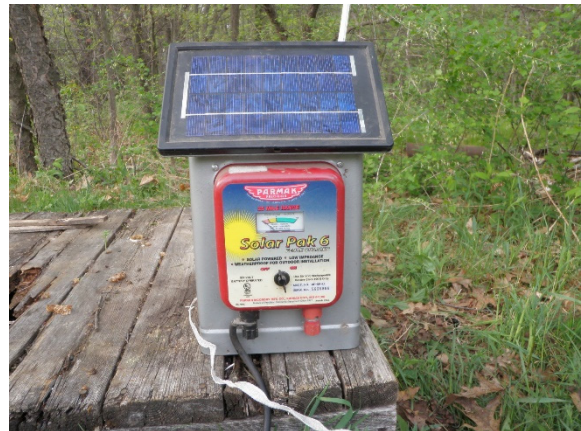
Figure 9. A solar-powered charger can provide electricity for a fence. Photo by Jan Hygnstrom.
