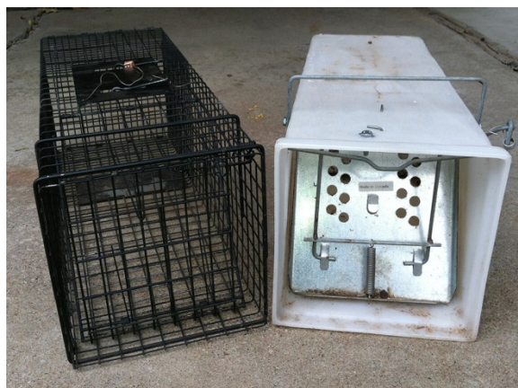
Figure 7. Cage traps have wire-mesh walls (left) while box traps (right) have solid walls. Photo by S. Vantassel.
