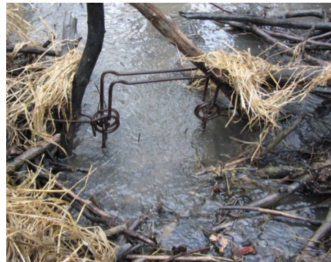
Figure 5. Conibear-style trap set in a beaver run set half-submerged with trigger on the bottom jaws. Photo by Stephen M. Vantassel.
