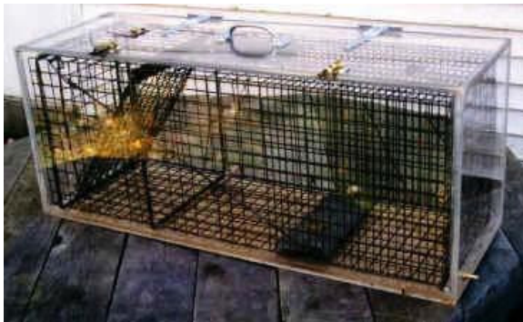
Figure 2. A cage trap enclosed in a carbon-dioxide euthanasia chamber constructed with Plexiglas®. Photo by Stephen M. Vantassel.
