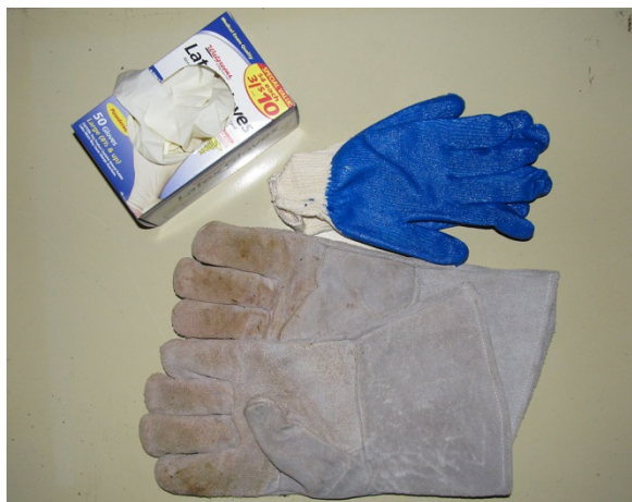
Figure 3. Top left and moving clockwise: Latex gloves, rubberized cloth gloves, and welder's gloves. Photo by Stephen M. Vantassel
