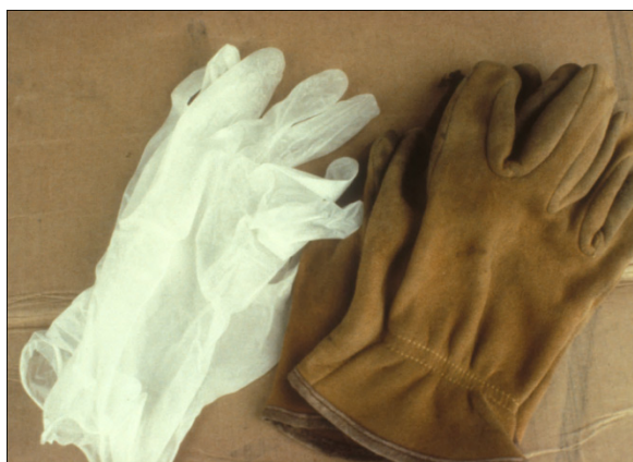
Figure 3. Plastic and leather gloves are essential safety items. Photo by University of Nebraska.
