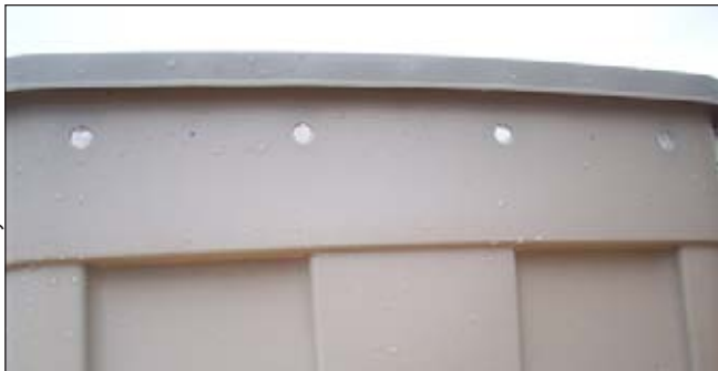
Figure 6. If commercial vents are not available, drill up to 10 ¼-inch holes on the sides, 2 to 3 inches below the lip of the tote. You can glue screen material to the holes to prevent fruit flies from invading the system.
