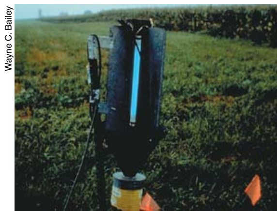
Figure 30. A blacklight insect trap uses a short-wavelength light to attract insects.
